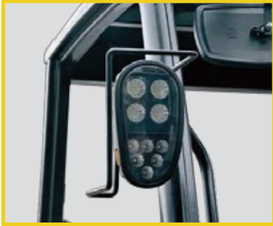
New LED lights provide superior and longer illumination whilst reducing energy consumption
